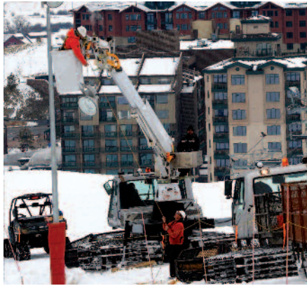
Left: A snowcat was fitted with a bucket for installation and maintenance. Right: A close-up of the bulb.
