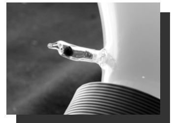
A small solid mercury amalgam ball is easily and safely snapped off for recycling. Magnets are recyclable metal and the remainder of the bulb is disposable glass.
